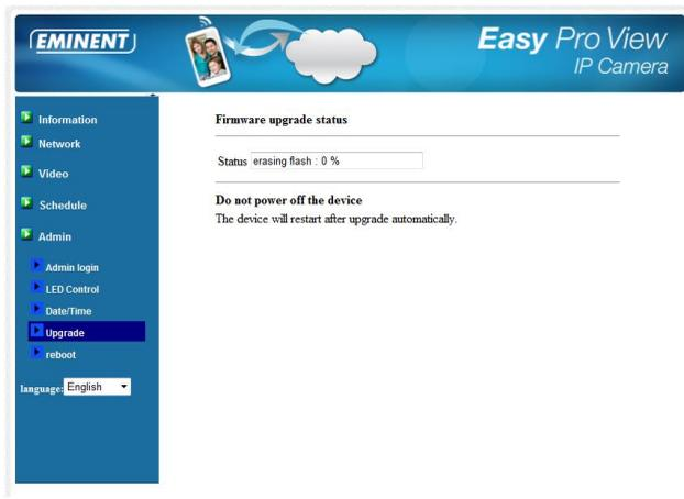
11. After successfully upgrading the Easy Pro View IP camera it will reboot automatically.
