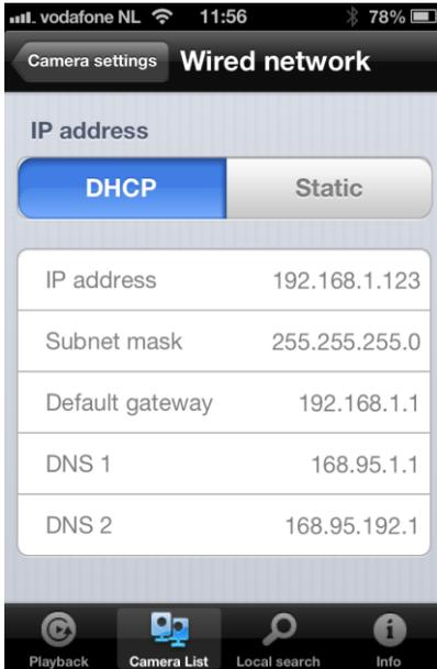
You can select if the camera will use a Dynamic (DHCP) IP address or a Static IP address (default setting is DHCP).
