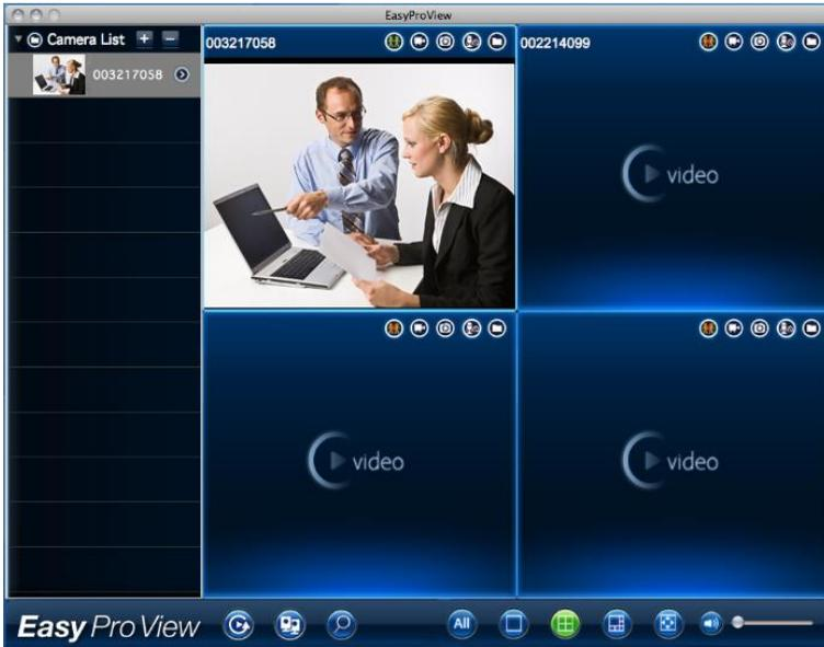
13. If the EM6250 is not in the same network as the computer you can add the EM6250 by clicking the **+** button next to the text "Camera List".
