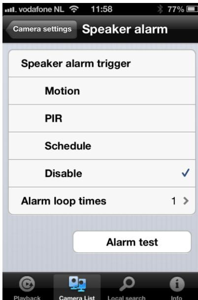
Select speaker alarm trigger and how many alarm loop times. Press Alarm test to test alarm (Please make sure a speaker is connected to the speaker jack).
