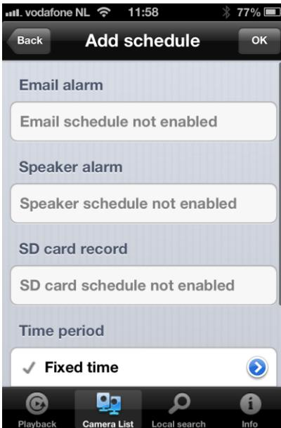
Select the trigger source: Email alarm, Speaker alarm, SD-Card record
