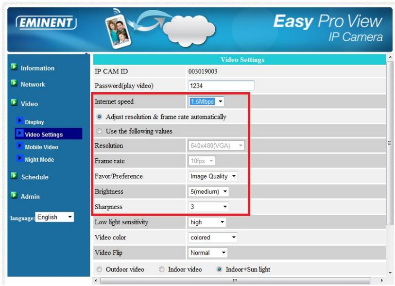
1. Internet speed – this is the Internet upload bandwidth of your network environment. Higher value will generate higher video quality and bandwidth. But if your Internet **upload** connection cannot provide more bandwidth than the specified value, the video quality could degrade and other devices using the same internet connection can experience connection issues. Please make sure to use a value that is lower than your internet upload bandwidth.
