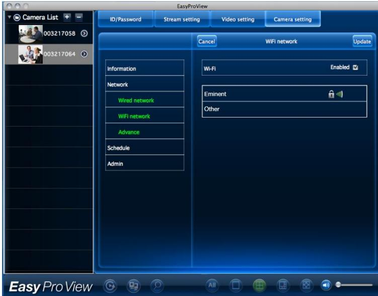
11. Now you can use 2 different ways to configure the camera to connect to the Wi-Fi network; manually or you can use the software to AutoDetect your Wi-Fi network.
